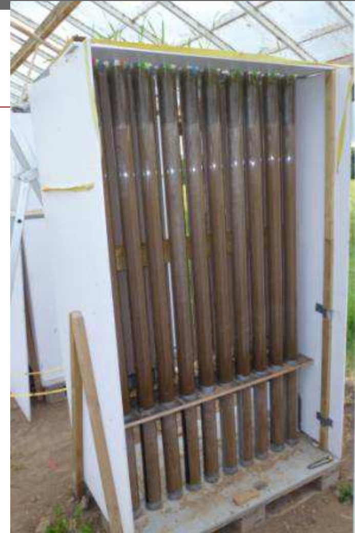
Root screening in aboveground Tube-Rhizotrons
